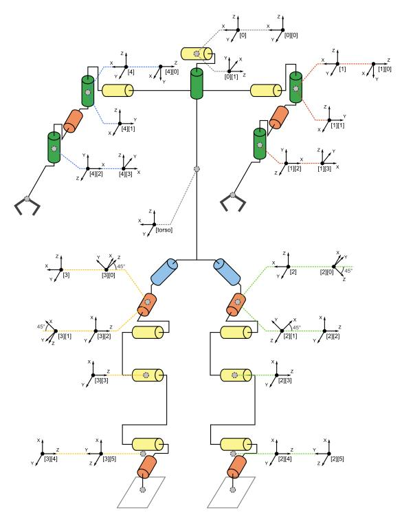
Figure 8.6: The joints of Nao robot.
