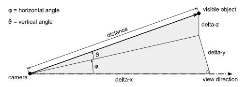
Figure 4.3: Polar coordinates as supplied by the 3D Soccer Server
