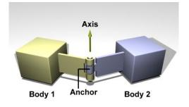
Figure 4.1: Hinge Joint ([Smi06])
