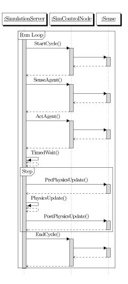
Figure 4.4: Single-threaded loop UML sequence diagram
