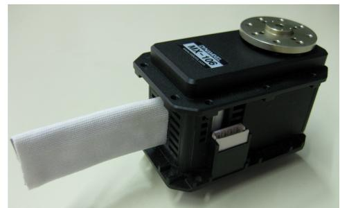
Fig. 6. Modified actuator with cooling fin.
